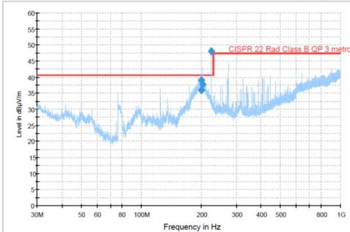
Figure 2: Radiated emissions, first equipment 2, before the modifications.
