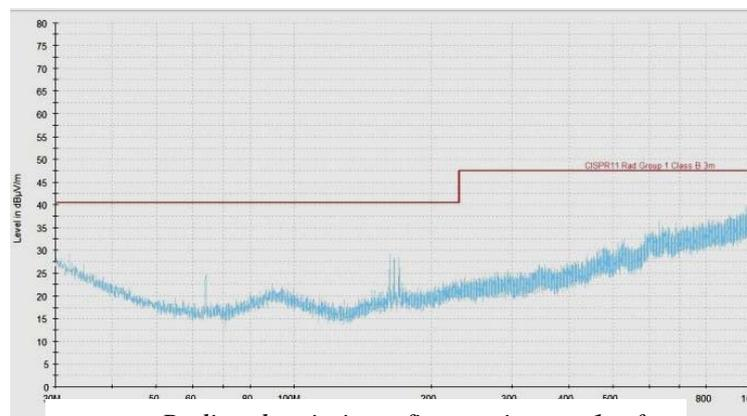
Figure 2: Radiated emissions, first equipment 1, after the modifications.
