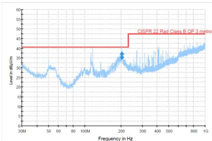
Figure 4: Radiated emissions, first equipment 2, after the modifications.
