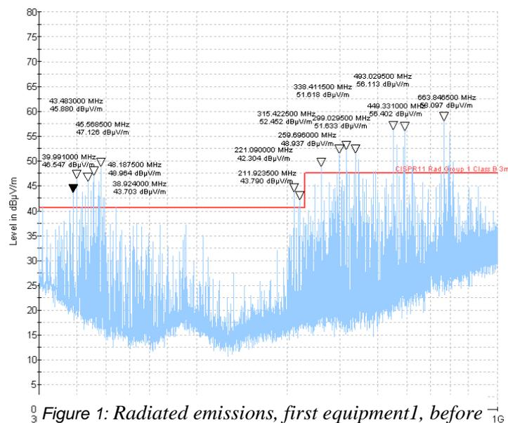
Figure 1: Radiated emissions, first equipment 1, before the modifications.
