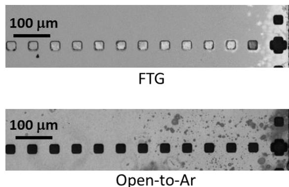
Figure 1. Optical microscope images showing the difference in EG near border regions of two samples processed together, (a) FTG and (b) open to Ar gas in the furnace.
