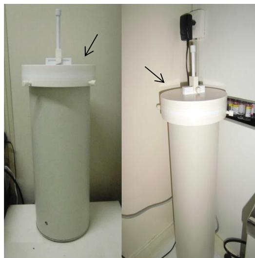
Figure 2: The black arrows show the device mounted on top of the both IC, demonstrating the fit and system functionality. The convenience and ease of handling device, allows the procedure to be performed in the activimeters origin sites.
