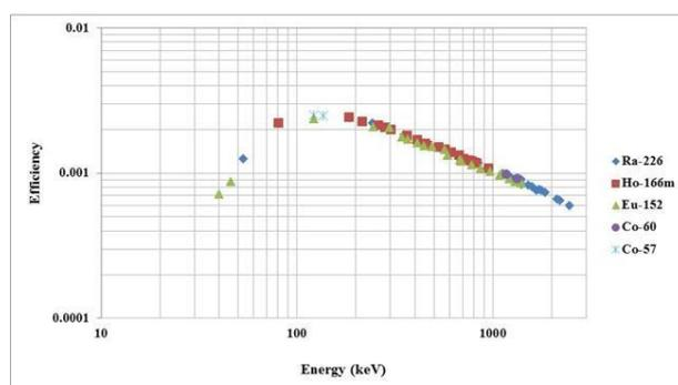
**Figure 3:** Efficiency versus energy calibration curve of germanium detector.
