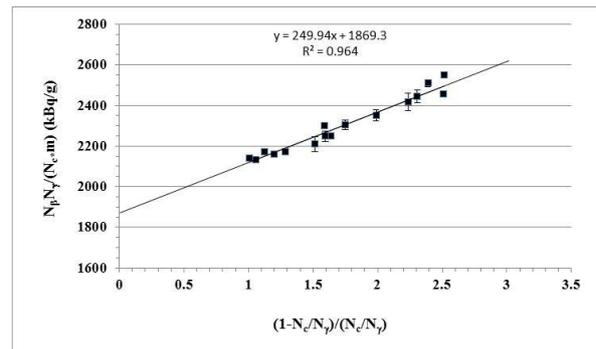
**Figure 1:** Typical extrapolation curve of experimental data for coincidence measurements of one source of  $^{201}\text{Tl}$ . The extrapolated value for  $(1 - N_c/N_g)/(N_c/N_g)$  gives the activity concentration of the source.
