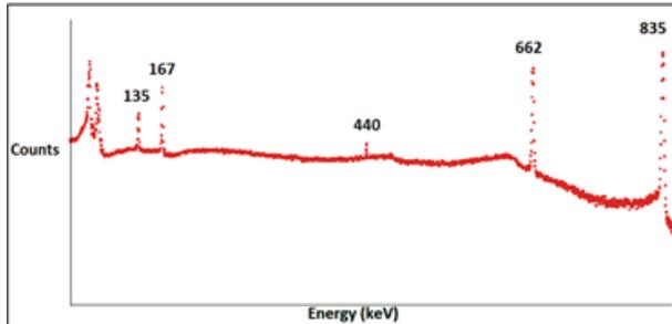
**Figure 4:** Gamma spectrum of  $^{201}\text{Tl}+^{137}\text{Cs}+^{54}\text{Mn}$  point source by germanium detector.
