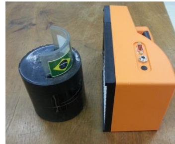
Figure 2. Calibration setup of the portable monitor using a Neck-thyroid phantom.
