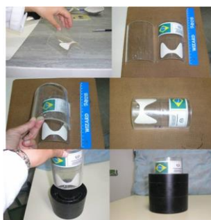
Figure 1. Neck-thyroid phantom developed at the In-Vivo Monitoring Laboratory of IRD [2].
