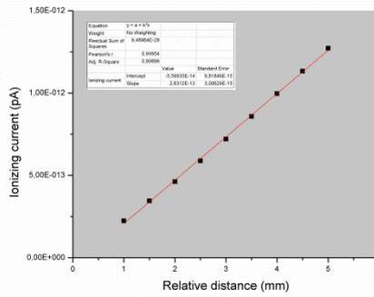
**Figure 4 Extrapolation line to determine the true null spacing ISO reference radiation N 30 Source : BASTOS, 2015**
