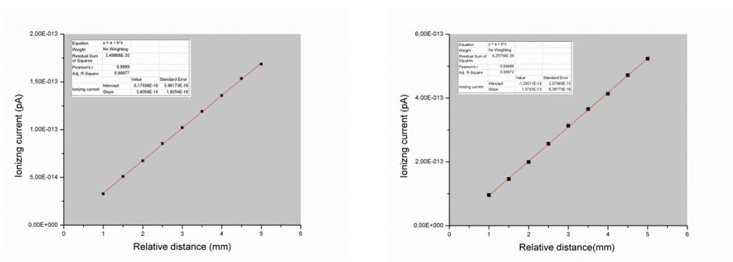
**Figure 2 Extrapolation line to determine the true null spacing. ISO reference radiation N 10 (Left side) and N15 (Right side) Source: BASTOS, 2015**
