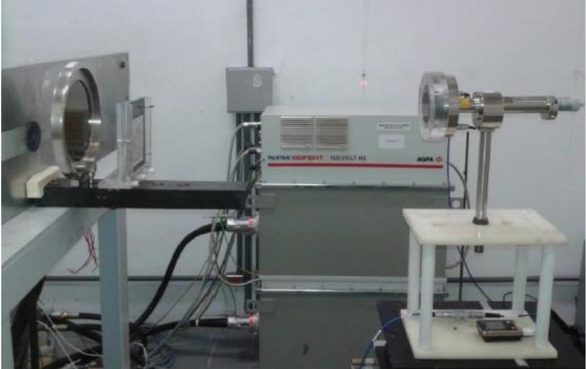
Figure 1 Experimental facility for determining the true null spacing of PTW 23392 extrapolation chamber for ISO series N.
