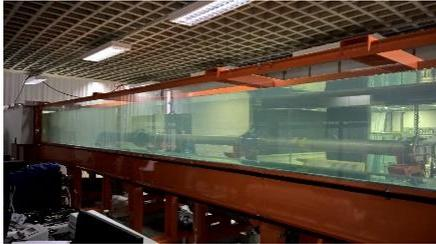
Figure 1 – The Circulating Water Channel – wide glass wall.
