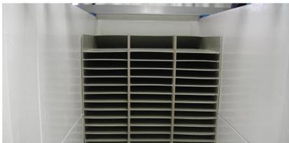
Figure 2 – Aspect of the flow straighteners.
