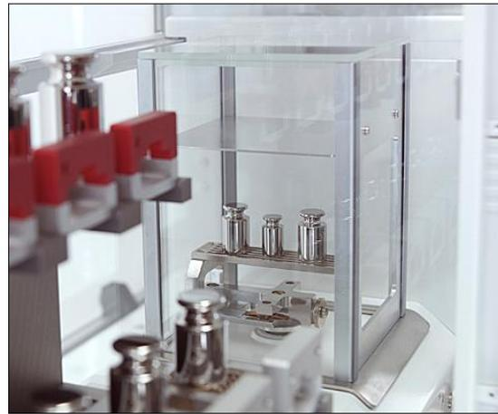
Figure 9. Three weights loaded symmetrically on the weighing pan of the a100 robotic comparator for dissemination.
