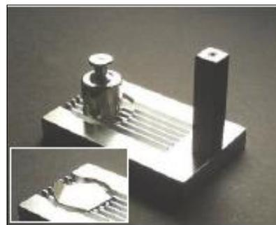
Figure 7. Weight carrier (1mg to 5g) of a5 robotic comparator.
