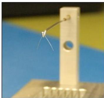
Figure 4. Weight with the nominal value of 0.05mg loaded on an a5 weight carrier.
