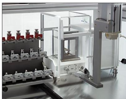
Figure 3. Robot switching dial weights of a100comparator.
