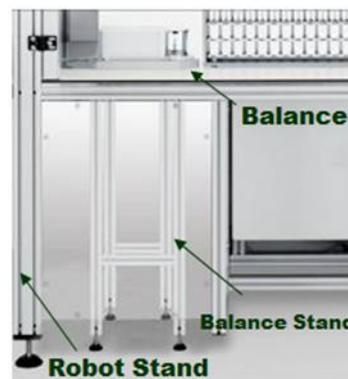
Figure 5. Separate stand of ultra-microbalance.
