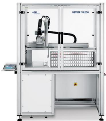
Figure 1. a5XL robotic comparator (0.05mg to 6g).
