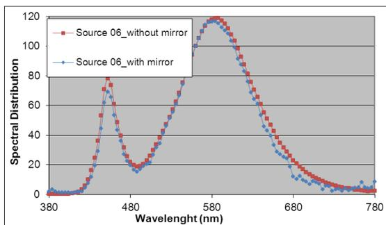
**Figure 5** - Measured spectral distribution from source 06 with and without mirror.
