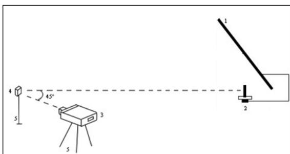
**Figure 1.** Setup without mirror reflection: 1: mirror; 2: lamp mounted on the goniophotometer arm; 3: spectroradiometer; 4: standard white tile; 5: tile mount and tripod.
