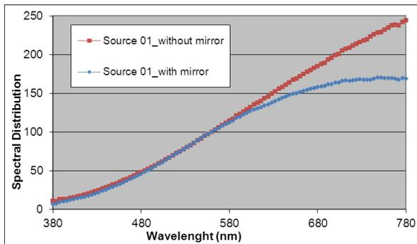
**Figure 3** – Measured spectral distribution from source 01 with and without mirror.
