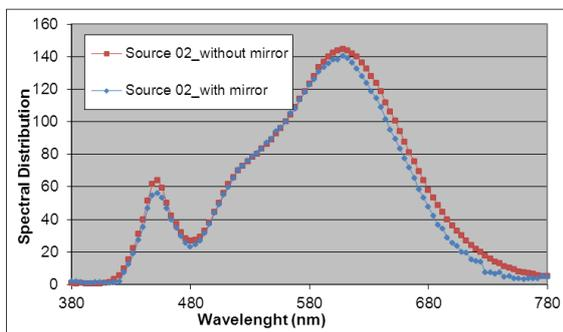
**Figure 4** - Measured spectral distribution from source 02 with and without mirror.
