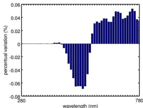
**Figure 2.** Percentual transmittance variation from 280 nm to 780 nm.
