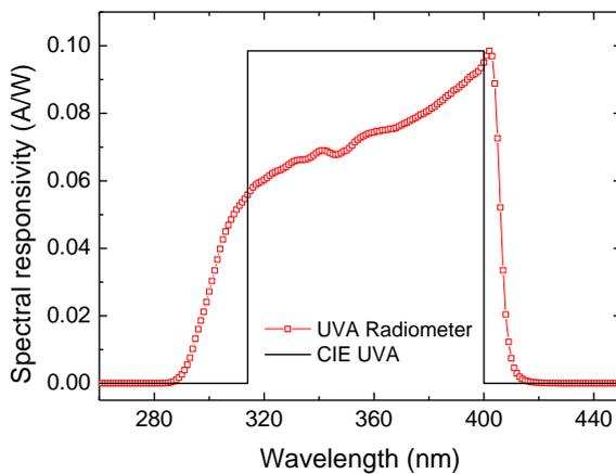
Figure 2 - Calculated spectral responsivity for the broadband UV radiometer alongside the CIE UV-A spectral function.
