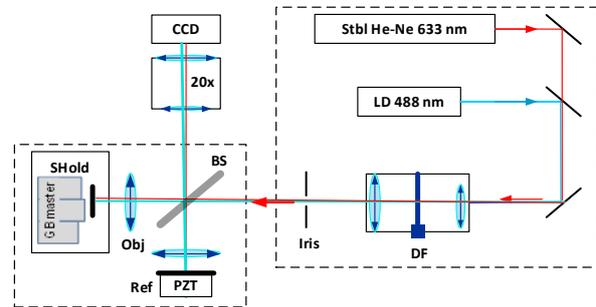
Fig.1. Optical setup of IM includes: **BS** - beam splitter, **SHold** - sample artifact on holder XYZ stage, **Ref** - reference mirror on PZT, **Obj** - two microscopic objectives, **DF** - rotating diffuser with beam collimator, **Iris** - variable diaphragm, **CCD** - imaging part with 20x zoom eye-piece.
