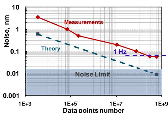
Fig.3. Stability of the measurement SHS 100 nm height deposited Aluminum (INMETRO).
