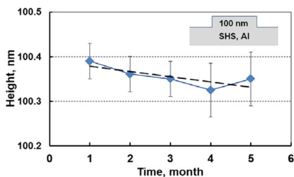
Fig.2 Drift of the measurement during several months. 100 nm SHS made of Aluminum.
