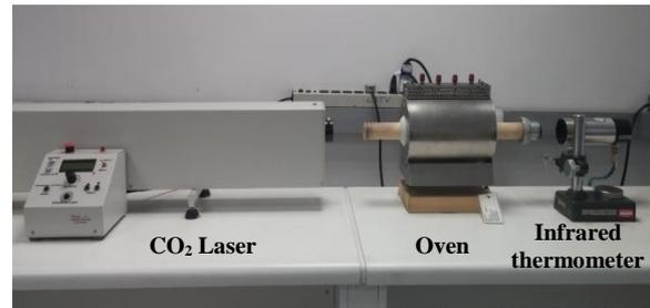
**Figure 1.** Apparatus for thermophysical properties measurements.
