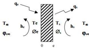
**Figure 2.** Heat transfer through a unidirectional plane wall.
