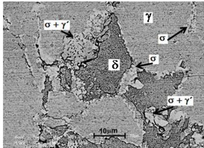
Figure 3. Micrograph of SAF 2205 steel treated at 800 °C for 2 hours obtained by SEM (Attack: Behara).
