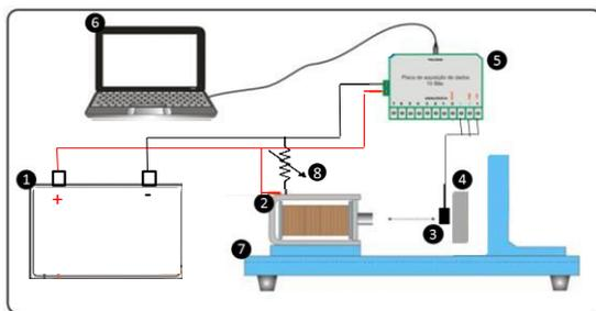
Figure 1. Experimental equipment of test: (1) Power supply; (2) Solenoid; (3) Hall sensor; (4) Sample; (5) Data acquisition board; (6) Computer; (7) Bench test; (8) Potentiometer.
