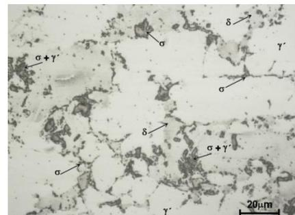
Figure 2. Micrograph of SAF 2205 steel treated at 800 ° C for 2 hours obtained by MO ( Attack: KOH ).
