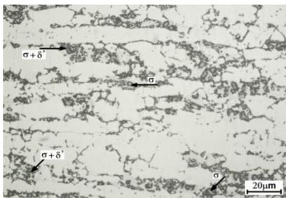
Figure 4. Micrograph of SAF 2205 steel treated at 900 °C for 2 hours obtained by MO (Attack: KOH).
