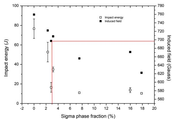
Figure 5 Change in absorbed energy and induced field due to the amount of sigma pass for a 10 V voltage.
