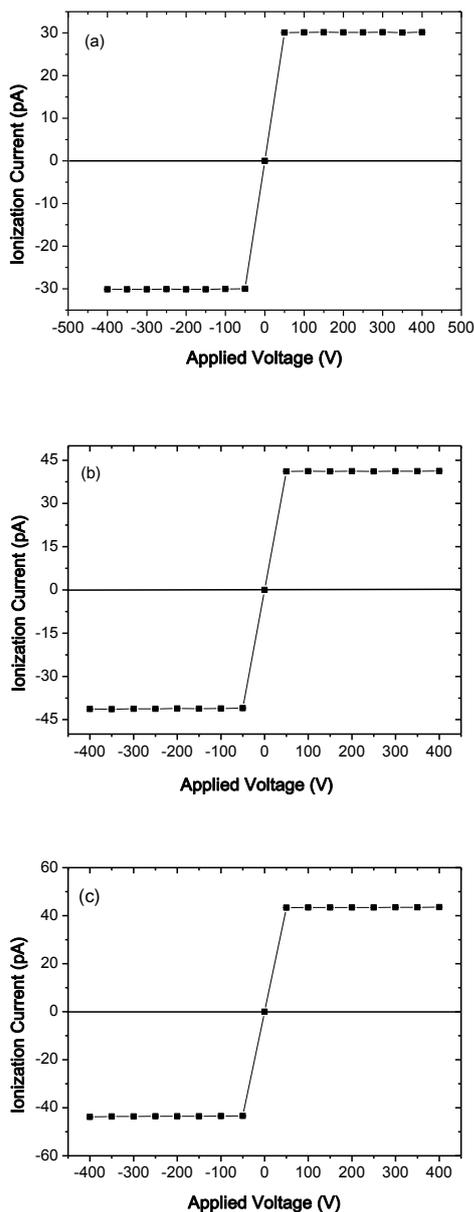
**Figure 1:** Saturation curves of the ionization chambers for the radiation quality RQT 9: (a) C1; (b) C2; (c) C3. The maximum measurement uncertainty was 0.59%.
