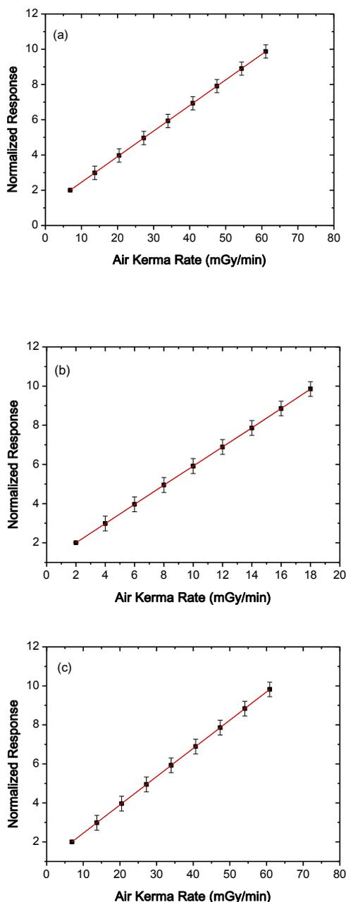
**Figure 2:** Linearity of response to quality RQT 9 of the ionization chambers: (a) C1; (b) C2; (c) C3.
