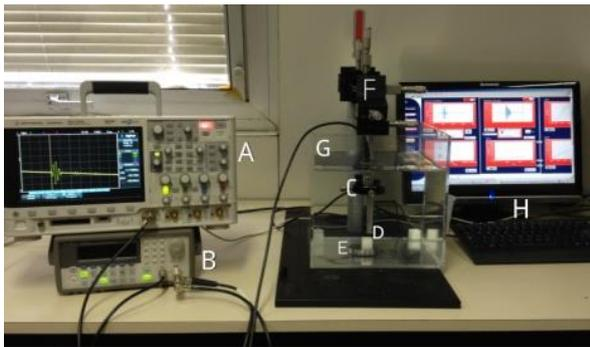
**Figure 2.** Measurement System: A- Oscilloscope, B- Arbitrary waveform Generator, C- Transducer, D- Bone replica sample, E- Reflector, F- Linear and angular stages, G- Water tank, H- Computer.
