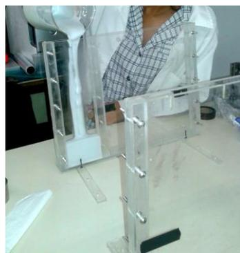
**Figure 3:** The mixture being poured into the mold.
