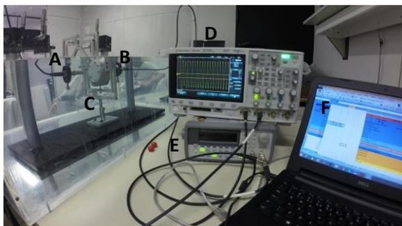
Figure 2: Experimental set-up for acoustic measurement. A, transmitting transducer with five degrees of freedom; B, receiver transducer with two degrees of freedom; C, specimen; D, oscilloscope; E, signal generator; F, computer.
