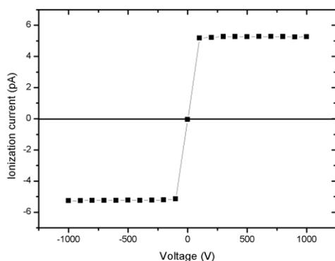
**Figure 2 - Saturation curve obtained of the free air ionization chamber in the collapsed position for the voltage in both polarities. The maximum uncertainty of the measurements was 0.5%, not visible in the graph.**
