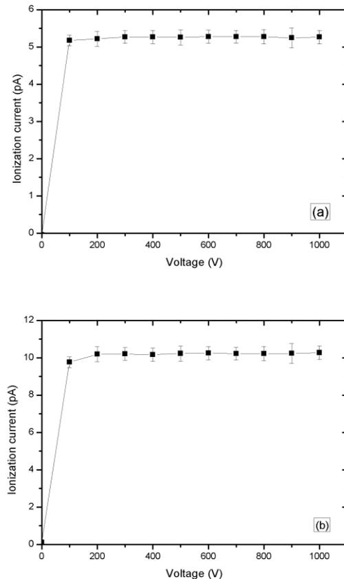
**Figure 1 - Saturation curves of the free air ionization chamber in the (a) collapsed position; (b) expanded position.**
