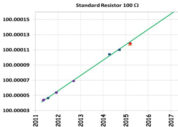
**Figure 7.** Historical evolution of 100  $\Omega$  standard resistor with two PTB sample calibrations (the two points to the right, red and orange).
