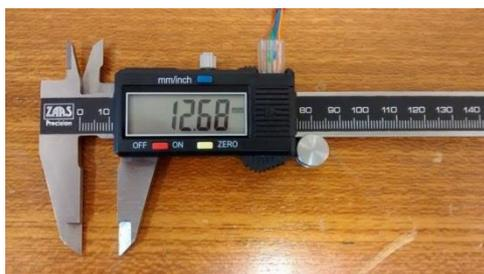
Figure 3. Digital caliper from Zaas company with conector. Source: author.
