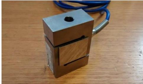
Figure 2. Load cell model CZCB-500. Source: authors.
