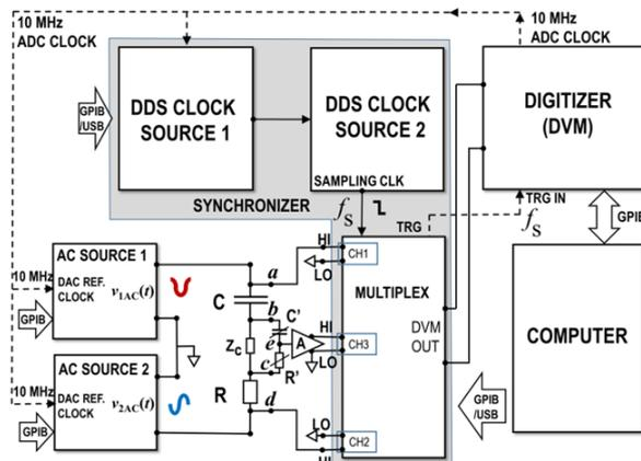
Figure 1 - Digital Bridge Diagram
