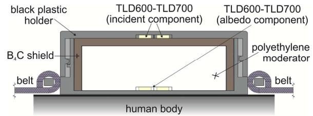
**Figure 1: IRD albedo dosimeter design.**
