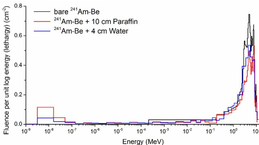
**Figure 3: Simulated moderated  $^{241}\text{Am-Be}$  neutron spectra compared to bare one.**
