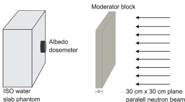
**Figure 2: Simulated irradiation geometry**
